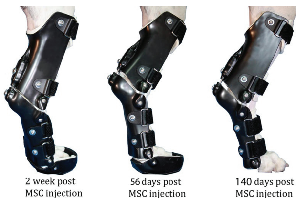
Figure 2 Custom, progressive, dynamic, orthosis used in the reported case. Initially, the talocrural and metatarsophalangeal joints were fixed at 165° and 75°, respectively. At 56 days posttreatment, 10° of extension was allowed in the talocrural joint. At 140 days posttreatment, the paw segment was removed.
