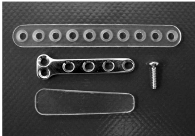
Fig 1. Biodegradable SR-PLA (70/30) plates and a metallic mini T-plate and 10 mm \times 2.0 mm miniscrew. The conical shaped SR-PLA (70/30) plate (bottom) was used for distal fractures. The mid-diaphyseal plate was similar to the straight commercial SR-PLA (70/30) plate (top), except there were no screw holes.
